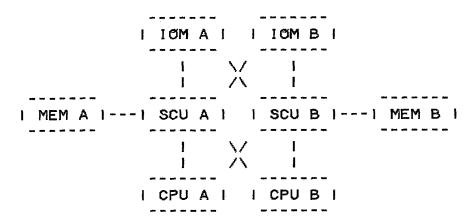
The crosses indicate that both IOMs and both CPUs connect to both SCUs; the CPUs and IOMs are not themselves connected.
